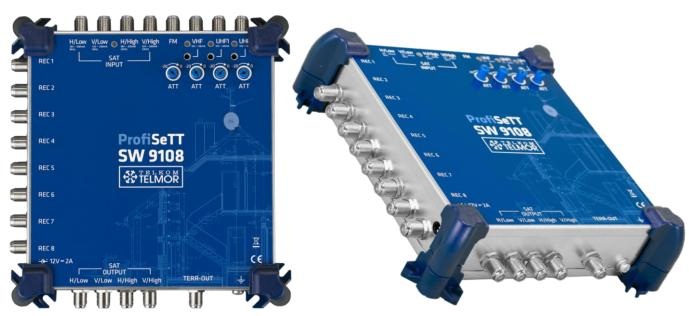
**SW-9108** is a solution that integrates the channel amplifier and legacy multiswitch in one housing. This allows to optimize installation costs and reduces the space requirement in the RTV-SAT distribution box. The device is dedicated to RTV-SAT installations in single-family houses.
